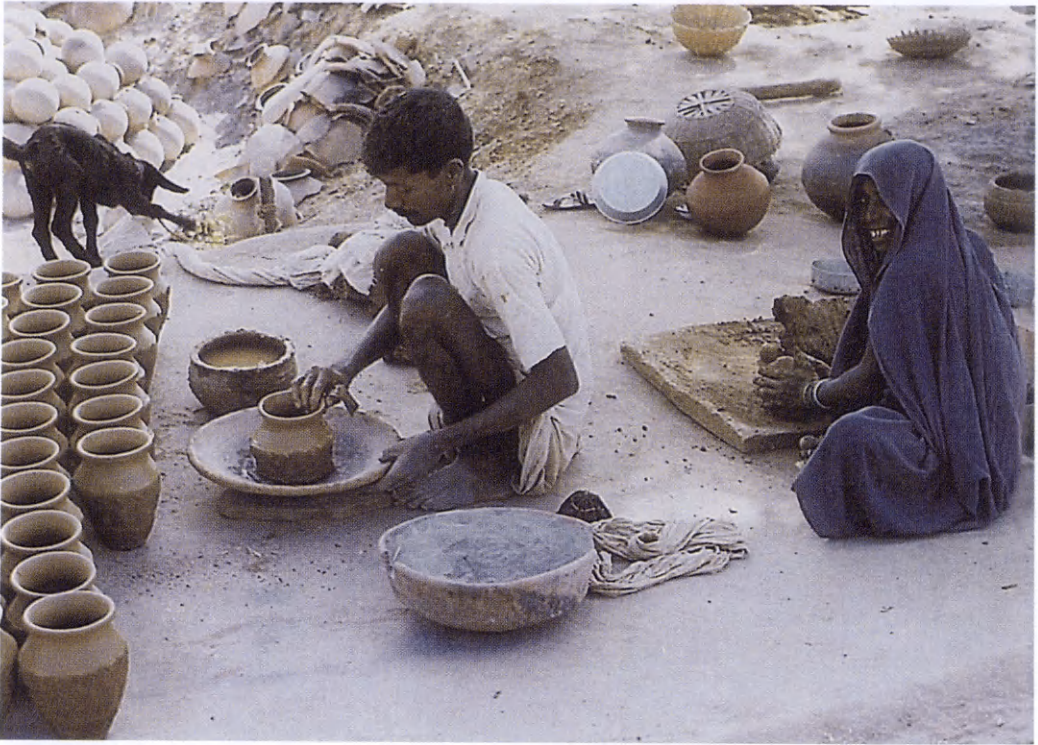
11. Handmade pottery workshop outside Kazuraho in India. Right: final kneading of the clay. Left: making the pot.
